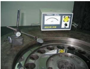
Figure 3: spindle axial displacement detection
