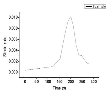
Figure 6: Strain rate of Max-Strain-Point VS time during drawing
