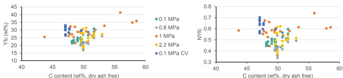
Figure 7: Experimentally achieved fixed carbon yields as a function of C content and pressure (CV: constant volume reactor, initial pressure) (Antal, 2000; Wang, 2016; Van Wesenbeeck, 2016; Legarra, 2018).
