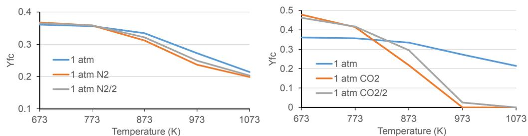
Figure 4: Fixed carbon yield as a function of temperature and carrier gas choice and amount (1 atm: no carrier gas, N<sub>2</sub> or CO<sub>2</sub>: carrier gas addition, N<sub>2</sub>/2 and CO<sub>2</sub>/2: halved molar addition of N<sub>2</sub> or CO<sub>2</sub>) at a pressure of 1 atm.
