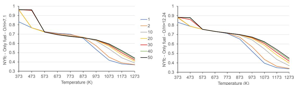
Figure 3: Normalised fixed carbon yield as a function of temperature and pressure (1-50 atm) for a constant carbon content in the feedstock, at an O/H ratio of 7.1 and 12.24.
