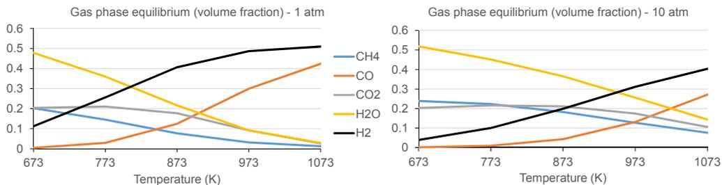
Figure 6: Gas phase equilibrium concentration as a function of temperature, at a pressure of 1 and 10 atm.
