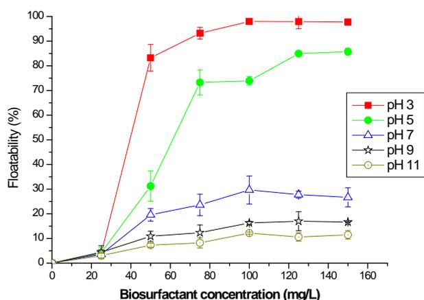
Figure 2: Floatability of hematite using the crude biosurfactant extracted from the *Rhodococcus erythropolis* bacteria as collector. Particle size: (<106  $\mu\text{m}$ , >75  $\mu\text{m}$ ); [NaCl]: 10-3 mol/L.
