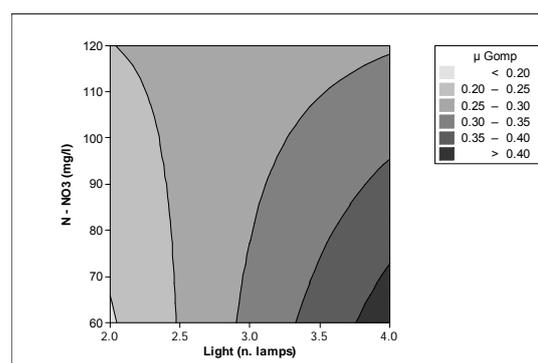
Figure 4: Interaction plot for Light and Nitrates, computed with  $\mu$  [day<sup>-1</sup>] as output
