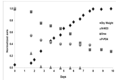
Figure 1: Dry Weight Vs. Urea, N- $\text{NO}_3$  and P- $\text{PO}_4$  consumption (Run 6 –  $t_0$ : Urea &  $\text{NO}_3$  120 mg/l)
