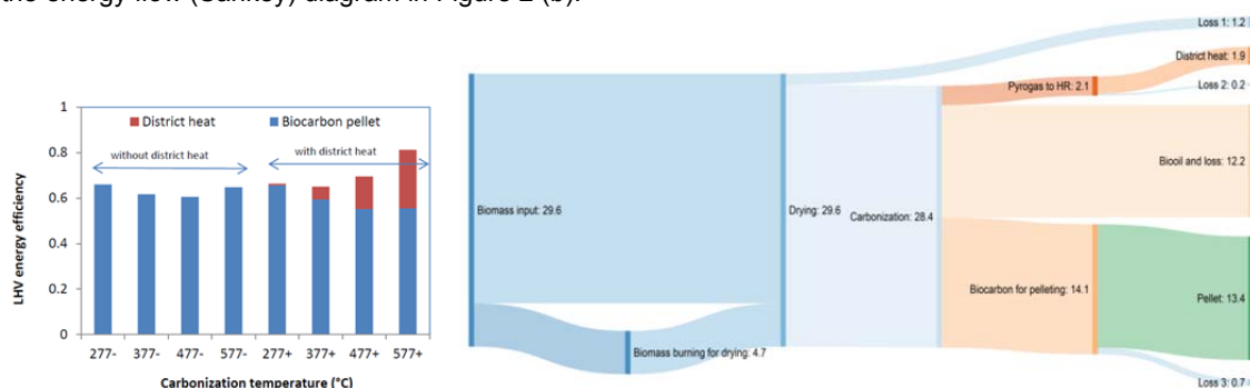
Figure 2:(a) Break down of LHV (lower heating value) energy efficiency in the case of biocarbon pellet production at various temperatures without (-) or with (+) coproduction of district heat (b) Sankey diagram for biocarbon pellet production at 477°C with district heat production, (Energy flow in MW).
