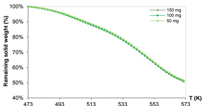
Figure 3: Evolution of solid weight versus temperature for different sample mass of commercial xylan from beech in TGA torrefaction experiments.
