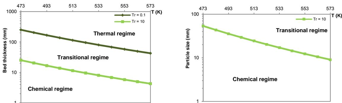
Figure 2: Torrefaction regime versus temperature and bed thickness (a, left) or particle size (b, right) for TGA.
