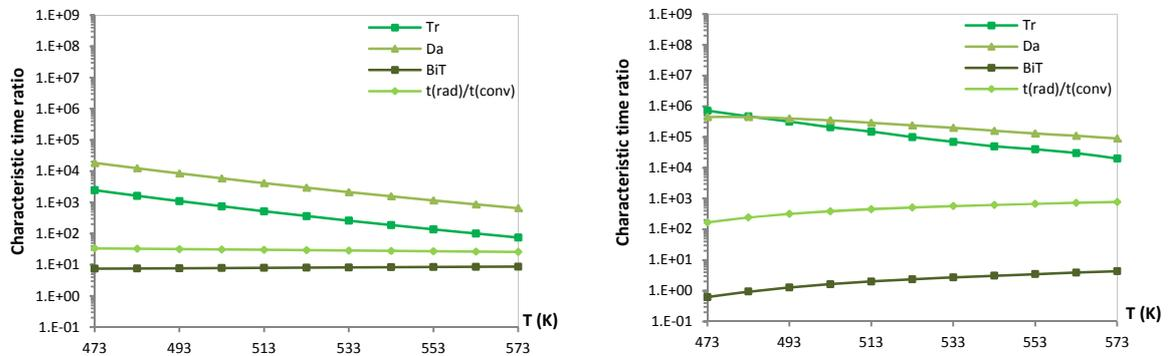
Figure 1: Dimensionless numbers ratio for bed-scale (a, left) and particle-scale (b, right) characteristic time analysis for TGA
