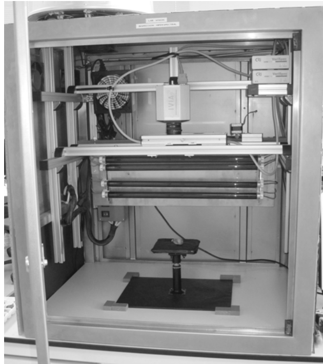
Figure 1. The hyperspectral system used for image acquisition
