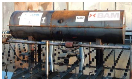
Figure 3: Bare Tank (no insulation or jacket) ready for test. Figure 4: Insulated and Jacketed tank ready for test.
