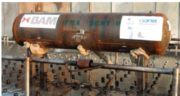
Figure 3: Bare Tank (no insulation or jacket) ready for test. Figure 4: Insulated and Jacketed tank ready for test.
