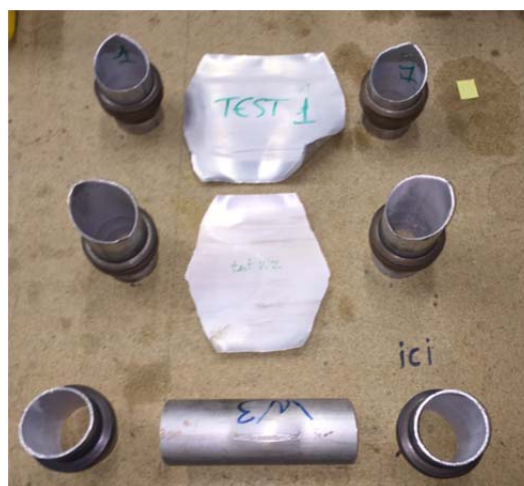
Figure 7: Sample views of failed vessel (BLEVE and non-BLEVE failures)
