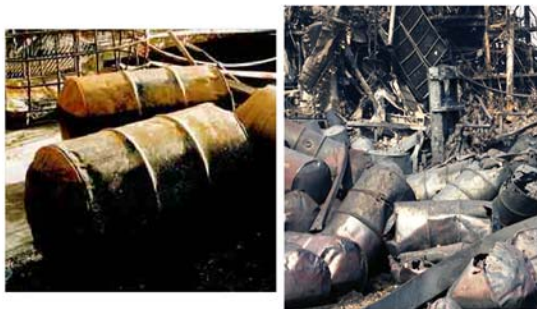
Figure 3: Observed damage showing the crushed pattern in oil drums in Flixborough (right) and Buncefield (left). Both sets of drum had been exposed to fire, the tell-tale stress mark showed that they had been exposed to high pressure compression loading.
