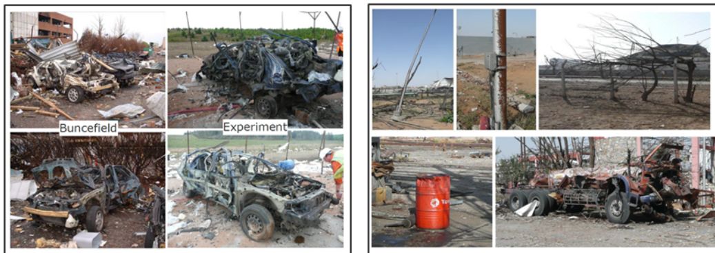
Figure 2: a (left) damage to car in the Buncefield incident and in experiments and 2b (right) directional indicators and pressure damage observed in Jaipur incident.
