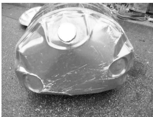
Figure 1: Blown up waste drum with dichloromethane, morpholine, methanol as main components. (Neuenfeld, 2008)
