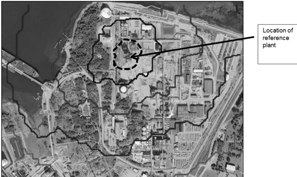
Figure 2: Individual risk contours for the design accident scenario, release of toxic gas. The dashed line represents 1.E-4 contour.
