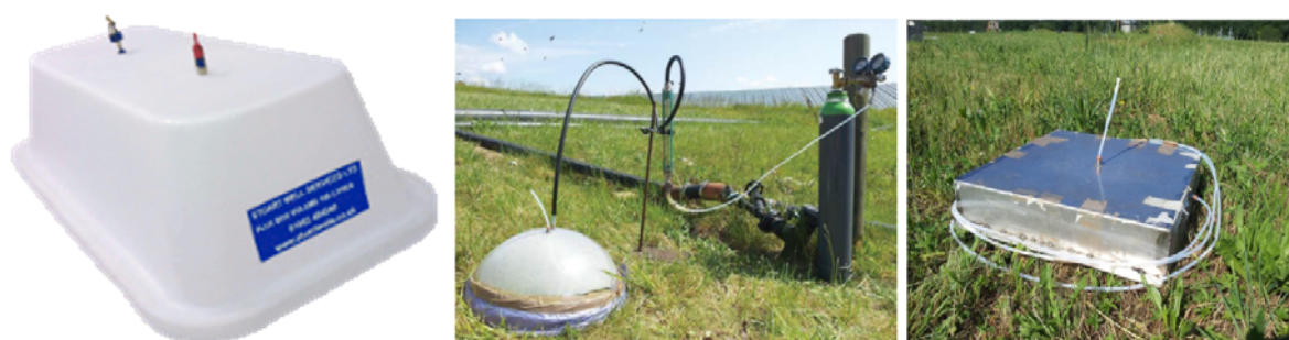
Figure 2: Examples of a static hood (left), a flux chamber (centre) and a device that can be operated both as static hood and flux chamber (right) for sampling on landfill surfaces
