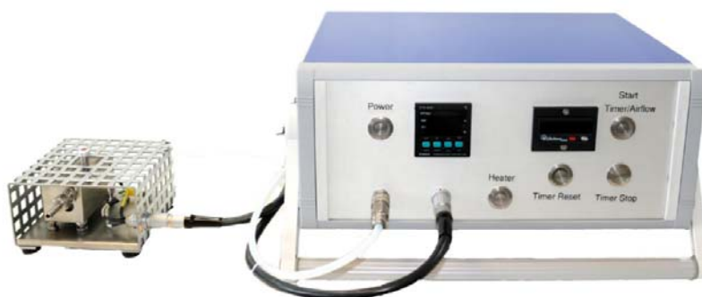
Figure 3: LiGaVa system consisting of a heating block and a temperature and air flow control element.
