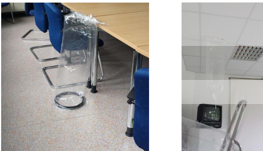
Figure 1: Sampling of floor (left), wall and ceiling (right) emission. Positioning of sample bags filled with cleaned air
