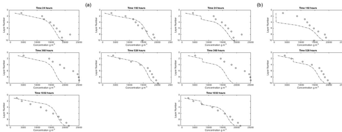
Figure 1: Solids profile concentration ( $g \cdot m^{-3}$ ) over time for the primary settler using: (a) Takacs et al. (1991) and (b) biological model. Dashed line (---) corresponds to model simulation and white circles (o) experimental data at 10 different depth points.
