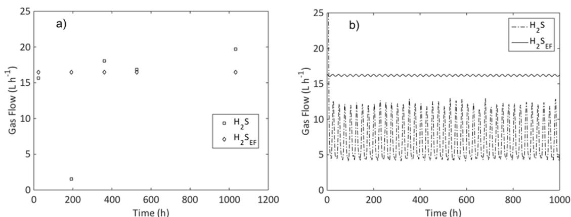
Figure 3: (a) Hydrogen sulfide air emissions flow rate from proposed dynamic model (□) and EF-based model (◇). (b) Simulation of the emission flow rates using white noise on model input variables compared proposed dynamic model (-.-) and EF-based model (-).
