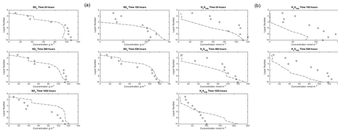
Figure 2: Sulfate (a) and hydrogen sulfide (b) water phase profiles concentration over time for the primary settler. Continuous line (-) corresponds to model simulation and white circles (o) experimental data at 10 different depth points.
