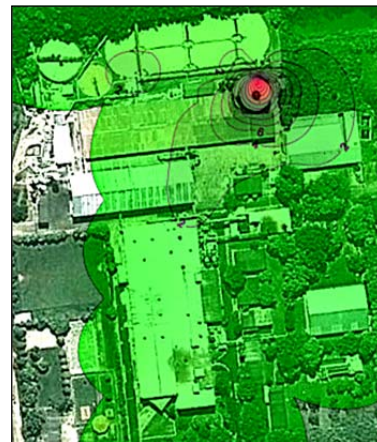
Figure 5: Chemical Industry and the H 2 S concentration plume (ppm) in extreme conditions - drain and sampling
