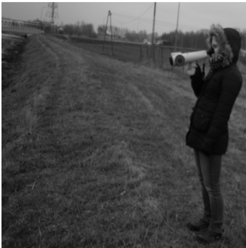
Phot. 1: Application of field olfactometer for measurement of ambient air with respect to odorants concentration in a vicinity of the sewage treatment plant of the LOTOS Group S.A. petroleum plant.
