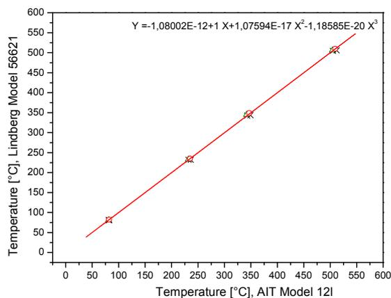
Figure 2: Temperature uniformity according to the Lindberg Model 56621
