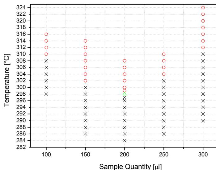
Figure 7: Ignition temperature at different sample volumes for 1-pentanol+water (circle: flammable case; cross: non-flammable case; triangle: the lowest flammable temperature)
