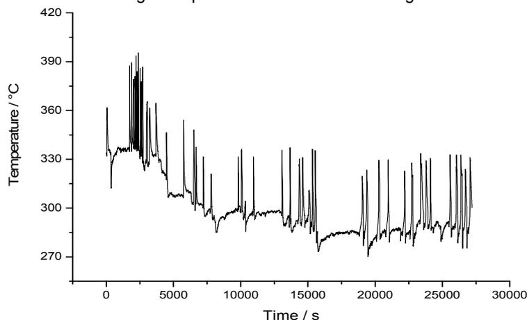
Figure 3: AIT owing to the 1-pentanol recorded at VEC, VSB-TU Ostrava
