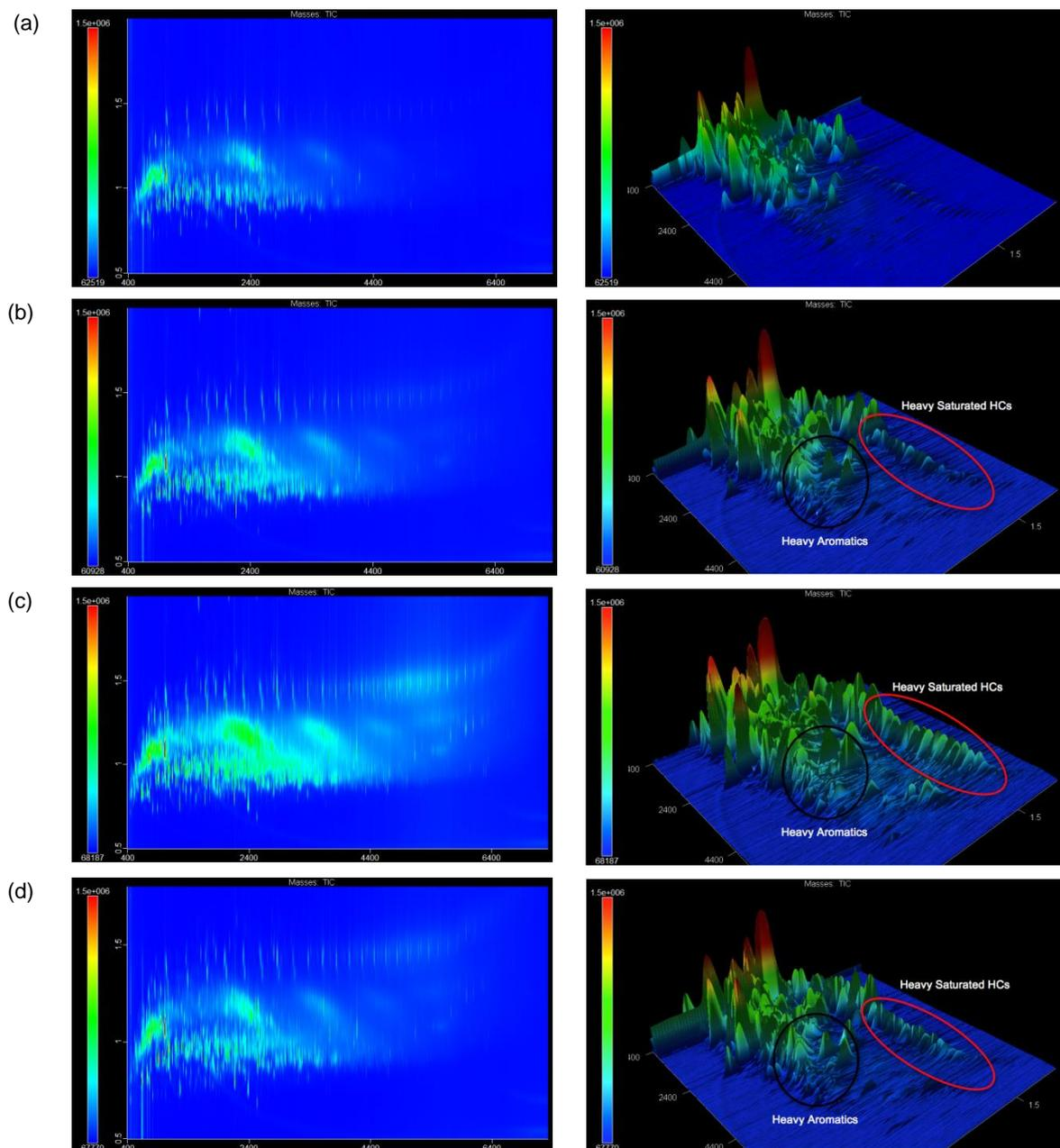
Figure 3: Contour plot and surface plot of total ion chromatograms: (a) untreated TDO (b) treated TDO with H<sub>2</sub>SO<sub>4</sub> (c) treated TDO with HNO<sub>3</sub> and (d) treated TDO with HCl
