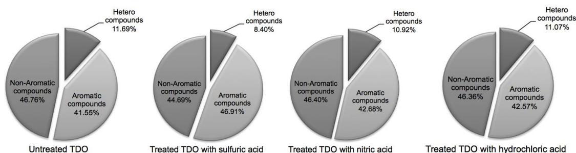
Figure 2: Contents of aromatics, non-aromatics and hetero compounds in tyre-derived oils.
