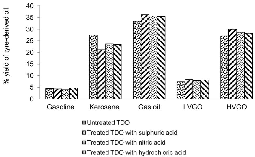
Figure 4: Petroleum fractions in maltenes of untreated and treated tyre-derived oils
