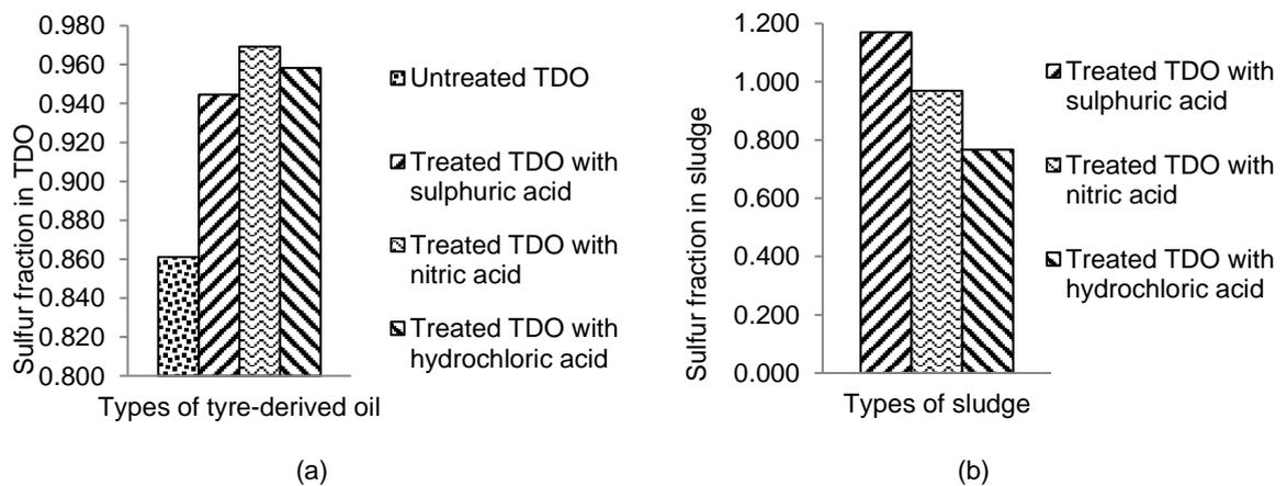
Figure 6: Sulphur content in products: (a) tyre-derived oils (b) sludge
