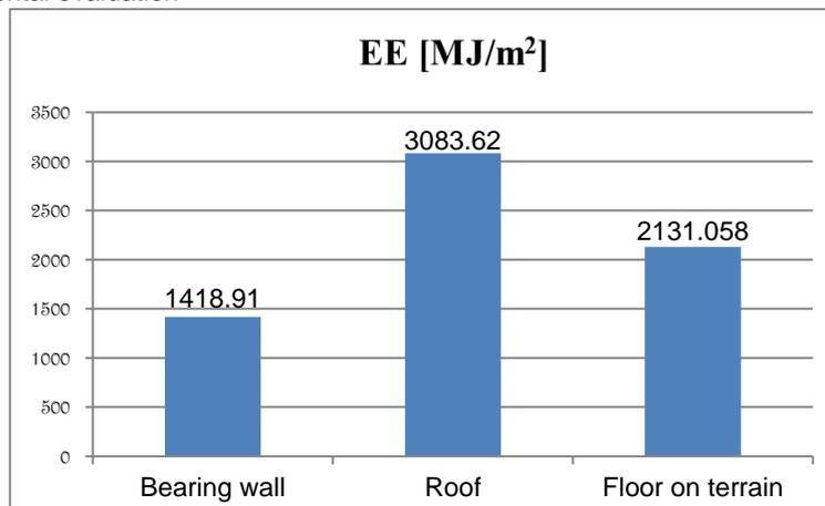
Figure 5: Embodied energy of building envelope constructions
