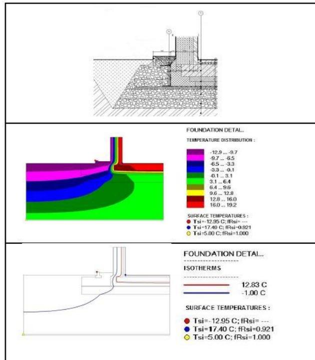
Figure 2: Thermo-physical evaluation of foundation detail in AREA Software
