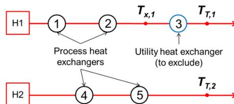
Figure 3: Example of the new features of the repair algorithm: utility exchanger 3 can be excluded from the formulation. The target temperature constraint for stream H1,  $T_{T,1}$ , is replaced by  $T_{x,1}$ .
