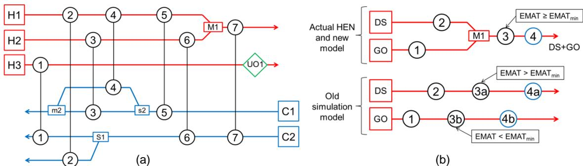
Figure 2: New types of splitters (S1) and mixers (M1) are considered in this work. *s2*, conventional splitter; *m2*, conventional mixer; *UO1*, simple unit operation; *DS*, diesel stream; *GO*, gas oil stream; *EMAT*, exchanger minimum approach temperature;  $EMAT_{min}$ , minimum allowed EMAT for the heat exchanger network.
