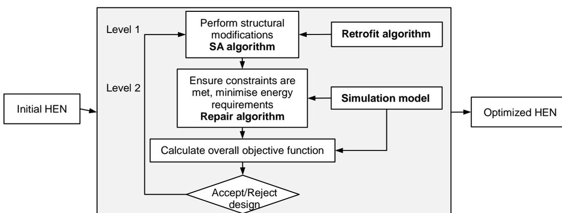
Figure 1: Two-level HEN optimization framework used in this work.
