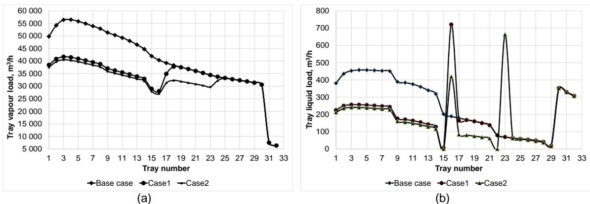
Figure 2: Tray loads of selected cases (a) vapour load, (b) liquid load
