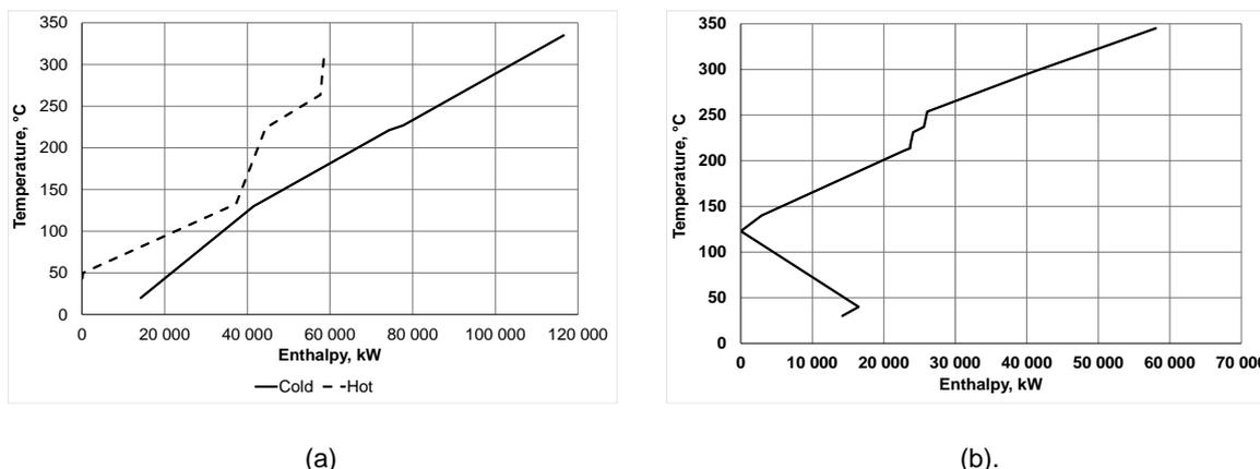
Figure 3: Composite and Grand Composite Curves for Case 1
