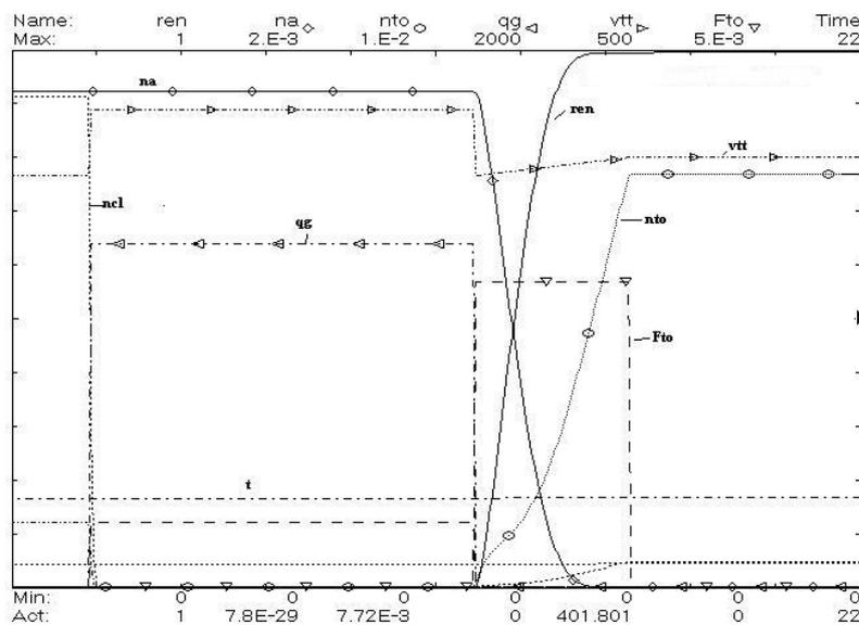
Figure 3: Performance of the process variables at different stage for the Reactor R-910. na: chlorates flow [kmol/h]; nto: thiosulfates flow [kmol/h]; qg: gases flow [m<sup>3</sup>/h]; ntt: total flow [kmol/h]; fto: feed flow of sodium thiosulfate [kmol/h]
