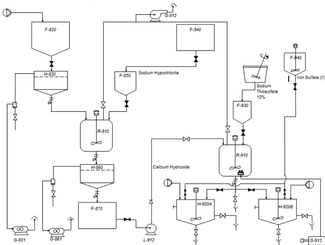
Figure 1: Technological scheme of the wastewater treatment plant.
