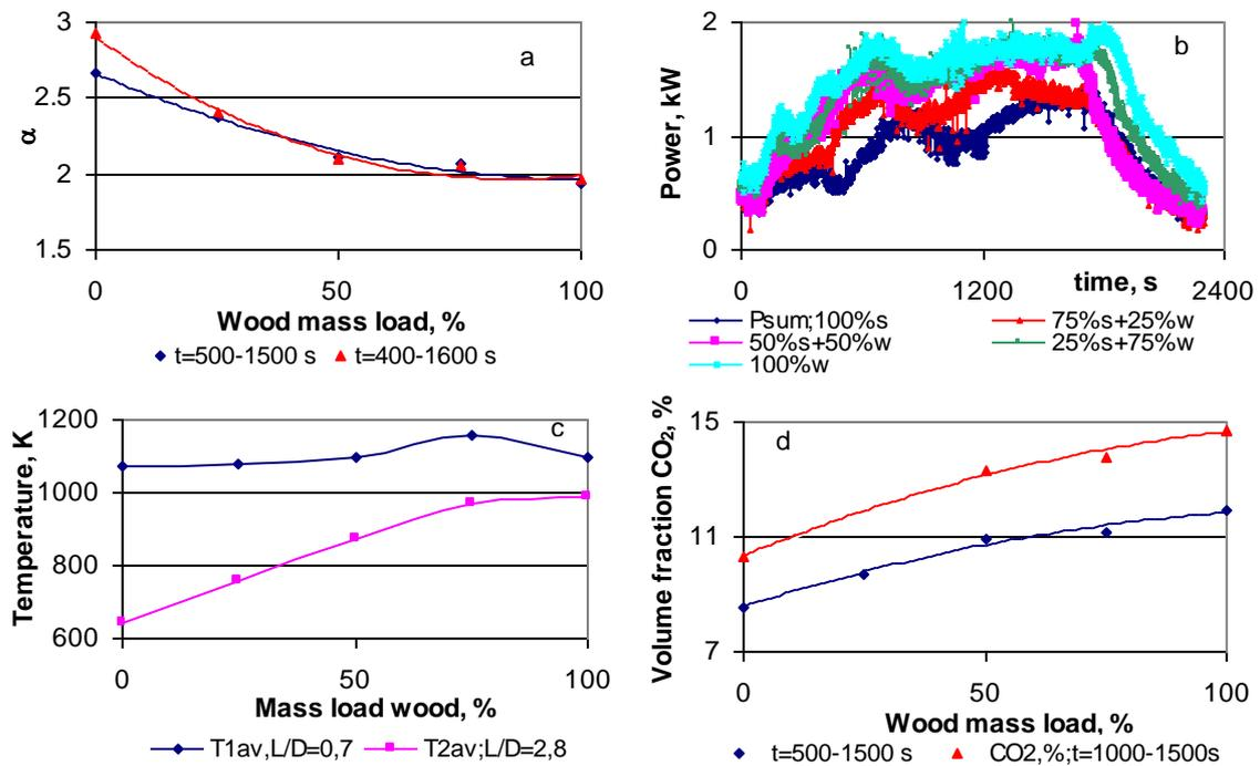
Figure 3: The wood mass load in the mixture with wheat straw pellets on kinetics of the heat output (a) and combustion characteristics (b-d).
