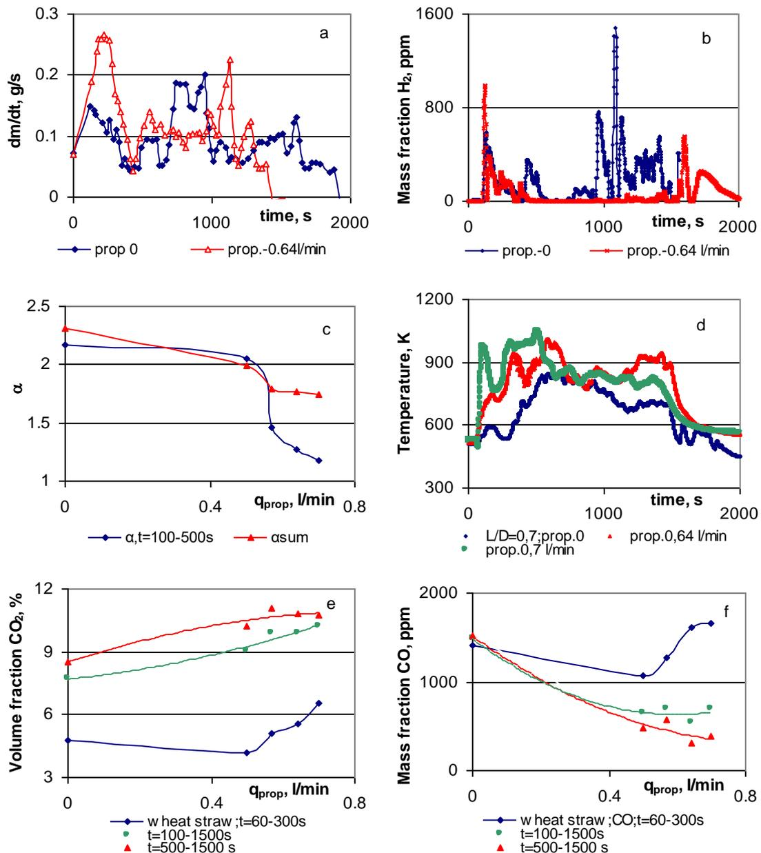
Figure 2: Effect of wheat straw pellets' co-firing with propane on the kinetics of the biomass weight loss rate (a), mass fraction of released  $\text{H}_2$  (b), air excess ratio in the reaction zone (c), kinetics of the flame temperature (d) and on the average values of the product composition (e, f).
