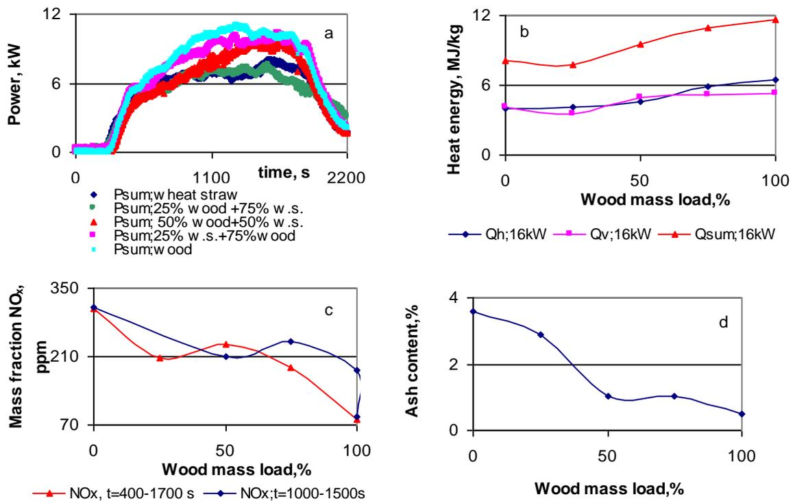
Figure 4: The wood pellets mass load on kinetics of a heat output (a), produced heat energy per mixture mass (b), mass fraction of  $NO_x$  in the products (c) and ash content (d).
