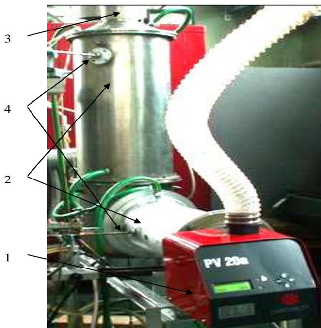
Figure 1: The technological device for experimental study of thermo-chemical conversion of biomass pellets; 1 - Pelltech burner, 2 - water-cooled sections of the combustor; 3 - chimney; 4 - openings for diagnostic tools.
