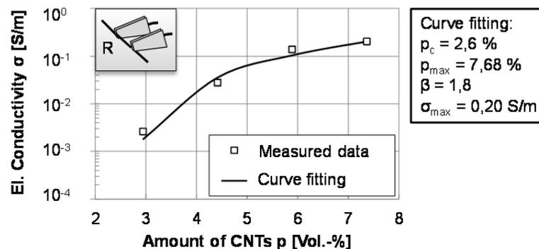
Figure 3: Electrical conductivity of the nanocomposite fibers as a function of CNT concentration
