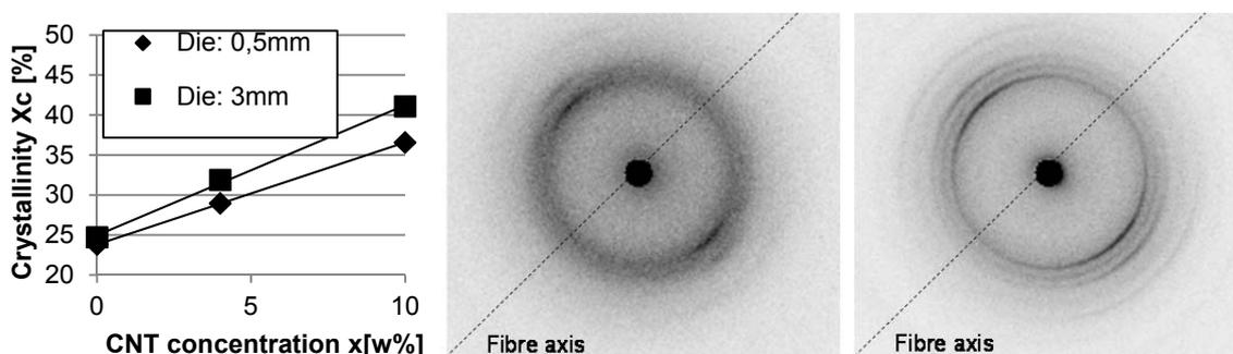
Figure 5: Crystallinity as a function of CNT concentration (left) and diffraction patterns of fibers with 0 w% (middle) and 10 w% CNT (right)
