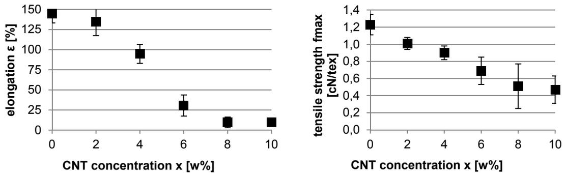
Figure 2: Mechanical properties of the nanocomposite fibers
