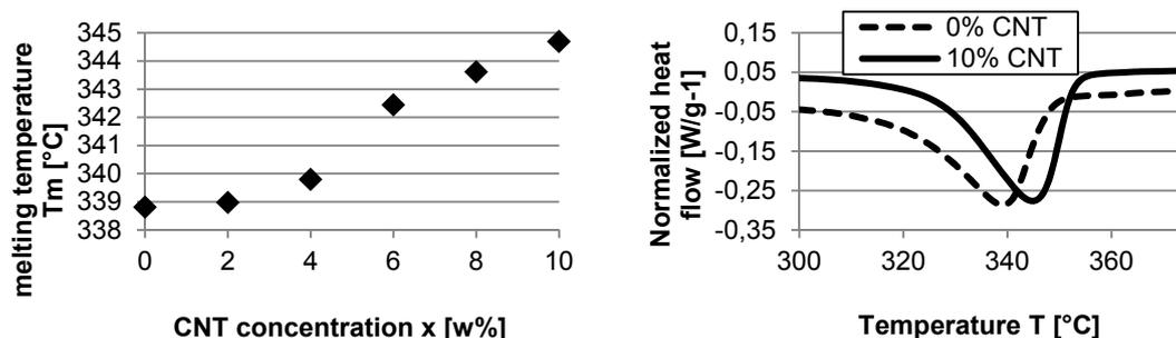
Figure 4: Melting temperature as a function of CNT concentration (left), DSC thermograms (right)
