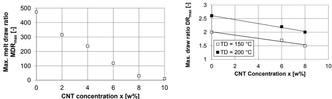
Figure 1: Results for processability to fibers as a function of CNT concentration, left: maximum melt draw ratio, right: maximum solid state draw ratio
