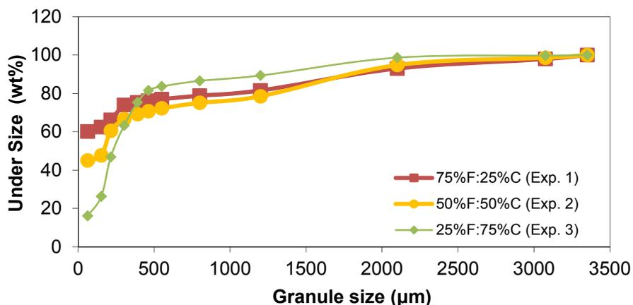
Figure 1: Granule size distribution at different powder ratio and constant 10 % of binder
