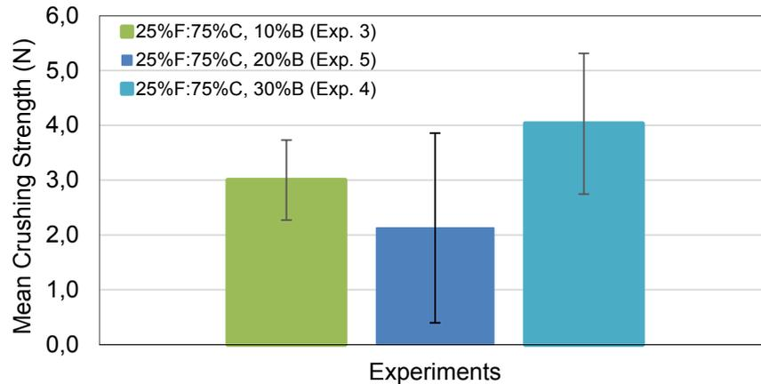
Figure 6: Mean crushing strength of 500 – 600  $\mu\text{m}$  granules at different binder percentage and constant powder ratio of 1/3 (25 % Fine: 75 % Coarse)
