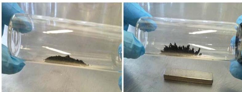
Figure 6. Photographs of G-FeCo nanoparticles: as prepared (a) and in response to Gd magnet (b).
