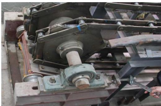
Figure 1: Transmission of Plate-Chain Conveyor
