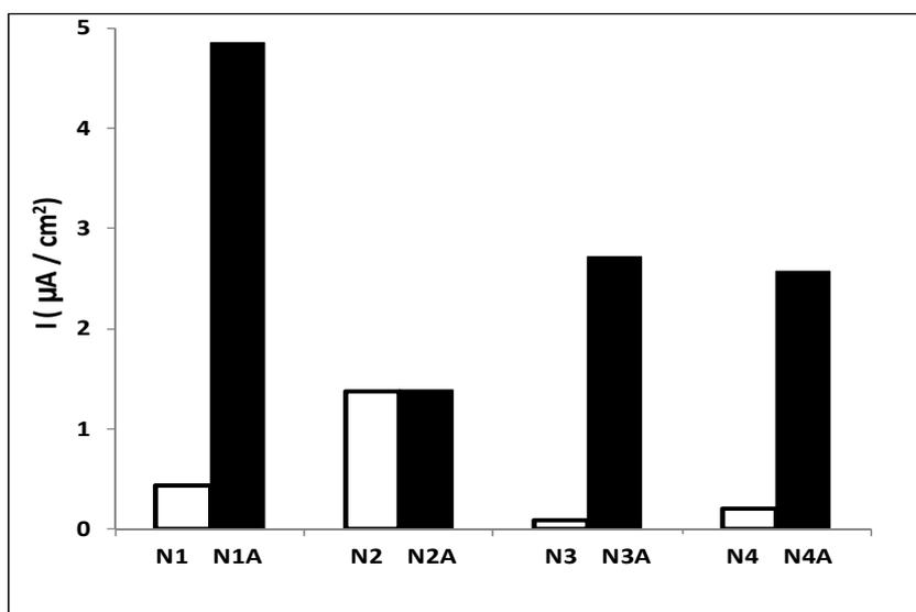
Figure 6: Photocurrent density of the bare Ni oxide and Ni/Al oxide films at 400 nm in 0.1M  $\text{Na}_2\text{SO}_4$ .
