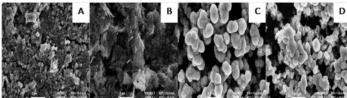
Figure 3: SEM images of the Ni oxide films: N1 (a), N2 (b), N3 (c) and (d) N4.
