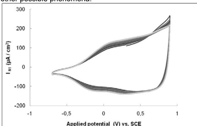
Figure 2: Repeated cycles of CV performed at N1 electrode in  $\text{Na}_2\text{SO}_4$  in the dark (scan rate:  $20\text{ mVs}^{-1}$ ).
