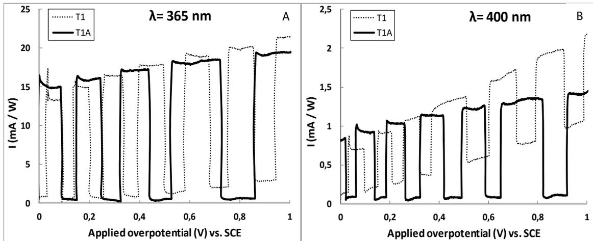
Figure 5: Normalized Photocurrent of T1 sample and T1A at 365 nm (a) and (b) 400 nm under chopped light irradiation in 0.1 M  $\text{KNO}_3$ .
