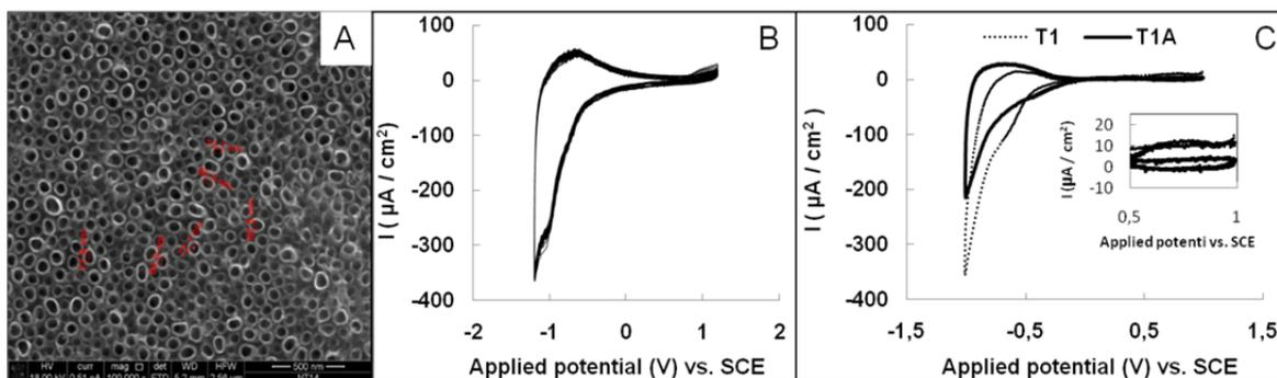
Figure 1: SEM images of the  $\text{TiO}_2$  NT structures (a); Repeated cycles of CV performed at T1 electrode (b) and (c) voltammograms obtained at T1 and T1A electrodes in 0.1 M  $\text{KNO}_3$  in the dark (scan rate:  $100\text{ mVs}^{-1}$ ).
