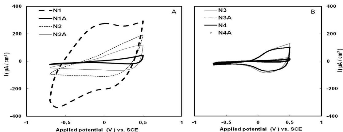
Figure 4: Voltammograms obtained at the N1, N1A, N2 and N2A (a) and (b) N3, N3A, N4 and N4A electrodes in 0.1M Na<sub>2</sub>SO<sub>4</sub> in the dark (scan rate: 20 mVs<sup>-1</sup>)
