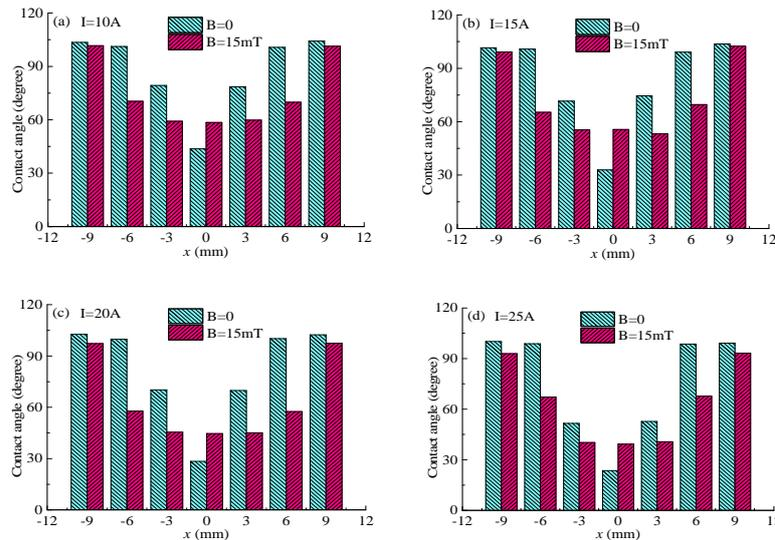
Figure 2: Contact angles distributions along x direction with different plasma arc currents
