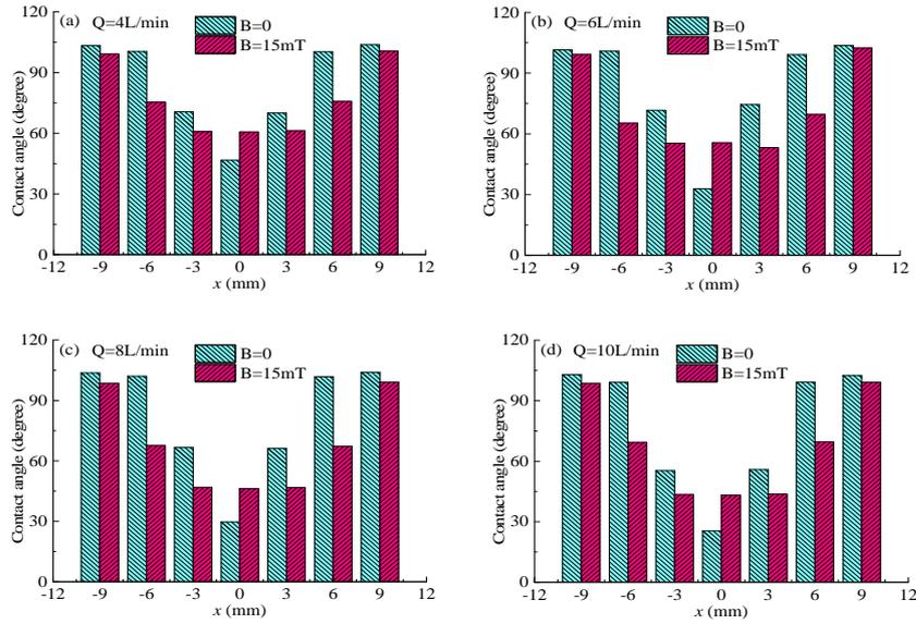
Figure 3: Contact angles distributions along  $x$  direction with different mixed gas flow rates
