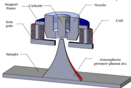
Figure 1: Schematic illustration of the cleaning system
