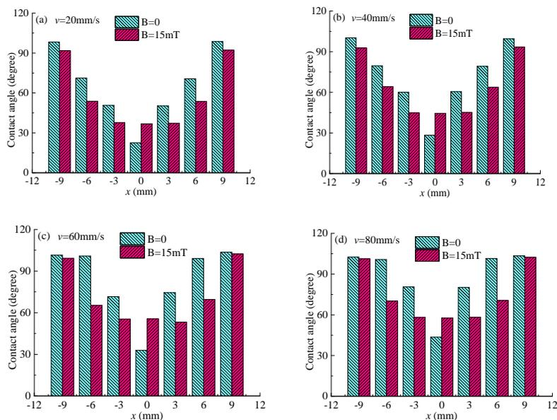
Figure 5 Contact angles distributions with different scanning velocity of plasma arc
