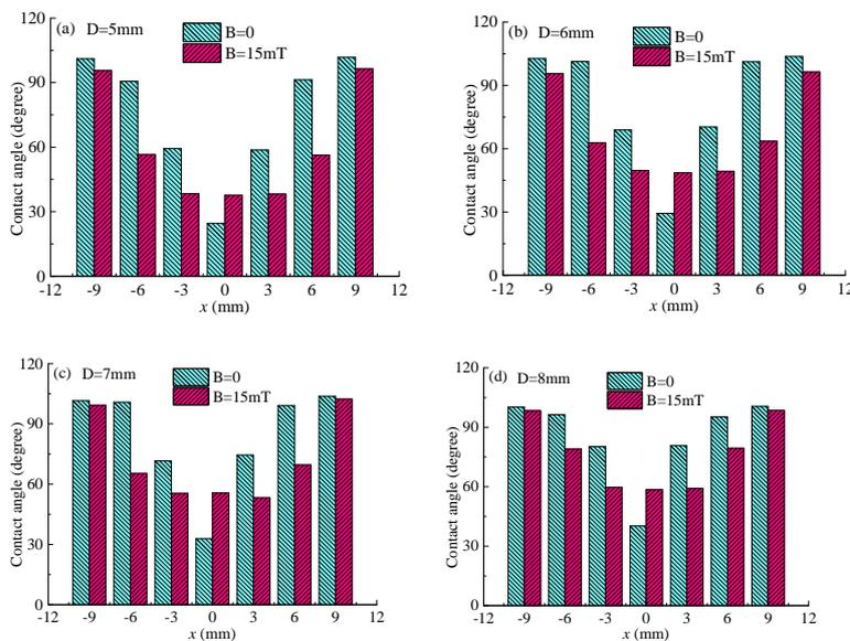
Figure 4 Contact angles distributions with different distances from the nozzle to sample surface
