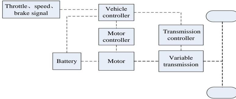
Figure 1: Transmission System Schematic Diagram
