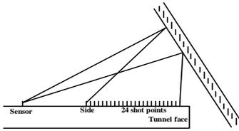
Figure 1: The advanced detection principle diagram of DTC-150
