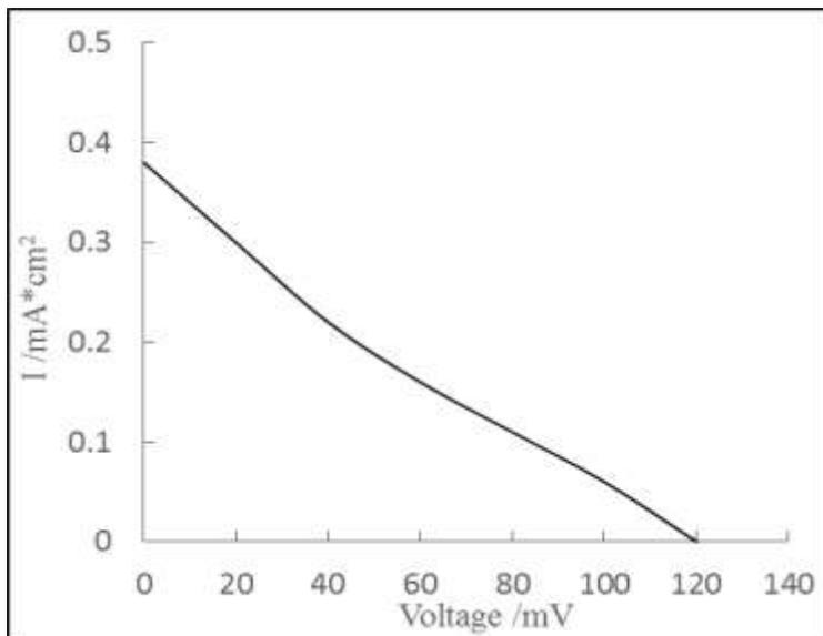
Figure 4: The I-V curve of SnO<sub>2</sub> sensitized by PbS quantum dot
