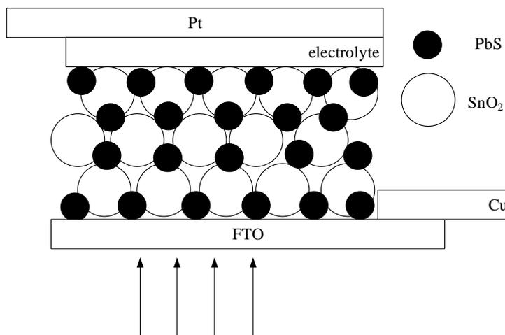
Figure 2: Assembly of the solar battery
