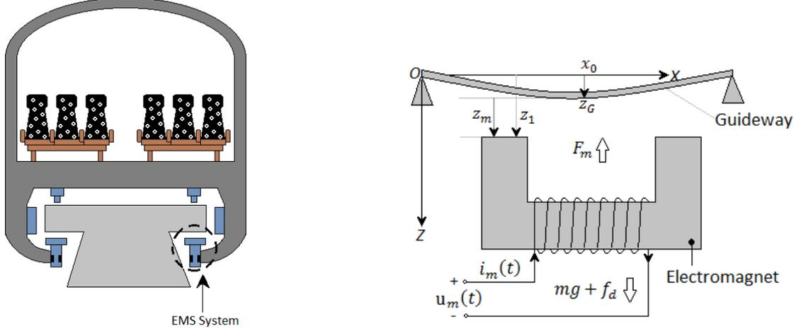
Figure 1: Structure of the MAGLEV train Figure 2: Basic structure of EMS module with flexible guideway
