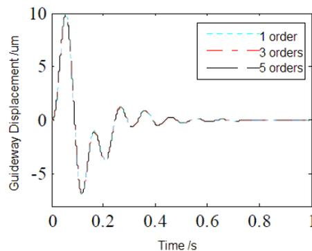
Figure 4: Vertical displacement of the guideway
