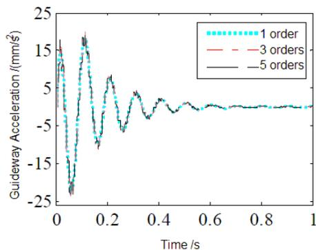
Figure 3: Vertical acceleration of the guideway
