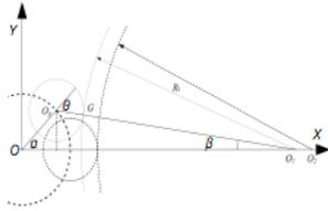
Figure 1: The schematic diagram of tangential point tracing grinding
