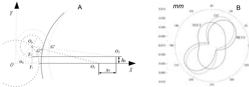
Figure 4: A) The combined effect of bigger grinding wheel radius and higher height B) The combined effect simulation of bigger grinding wheel radius and higher height
