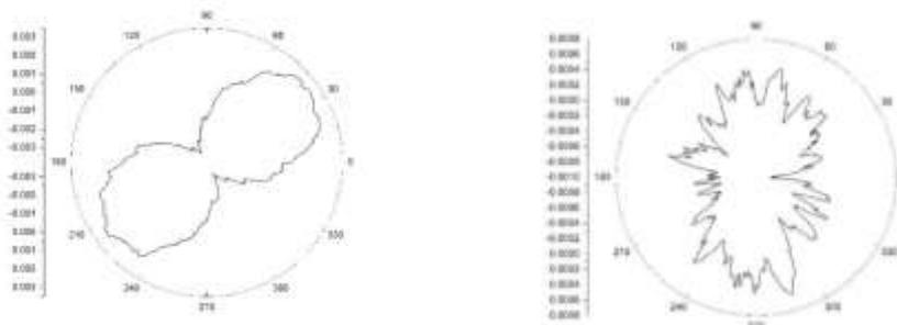
Figure 6: A) The sample roundness without error compensation B) The roundness with compensation
