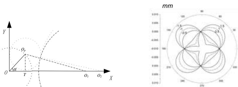
Figure 3: A) The grinding diagram with larger wheel radius than theoretical radius B) The crankpin roundness based on different grinding wheel radius errors
