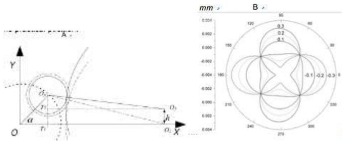
Figure 2: The grinding diagram with grinding wheel height error A) The grinding diagram with higher wheel height B) The crankpin roundness based on different grinding wheel height errors
