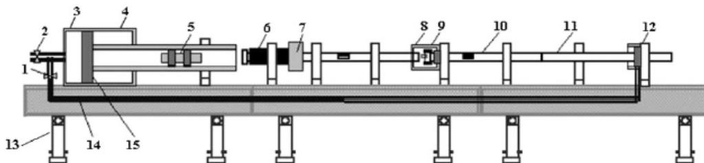
1- Exhaust valve; 2- intake valve; 3- back cavity; 4- front chamber; 5 - hitting rod; 6- input rod; 7- reaction bodies; 8- furnace and thermocouples; 9-specimens; 10- output rod; 11- absorbing rods; 12- drive; 13- supports; 14- air pipe; 15- pistons.
