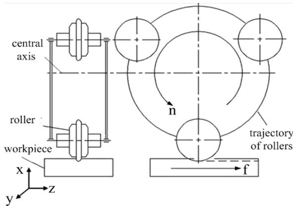
Figure 1: Principle of cold roll-beating forming
