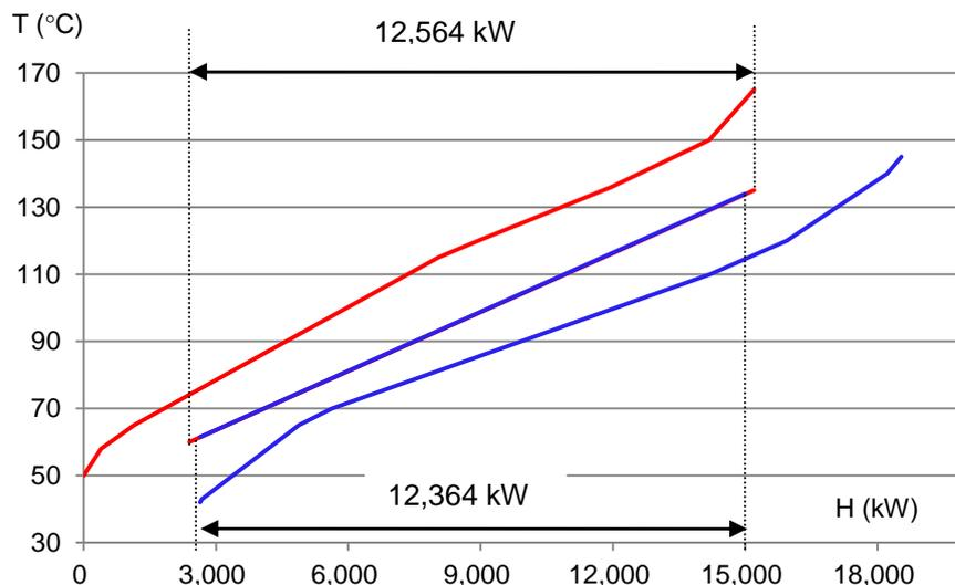
Figure 4: Composite Curve and intermediate fluid T-H profiles of Heat Integration
