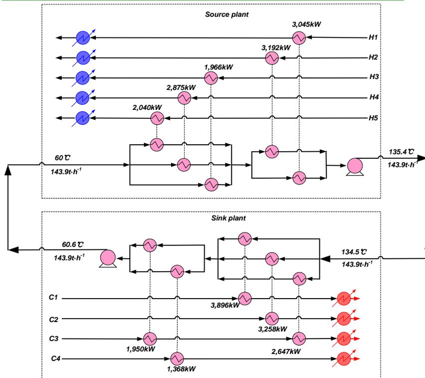
Figure 3: The heat exchanger networks in source and sink plants
