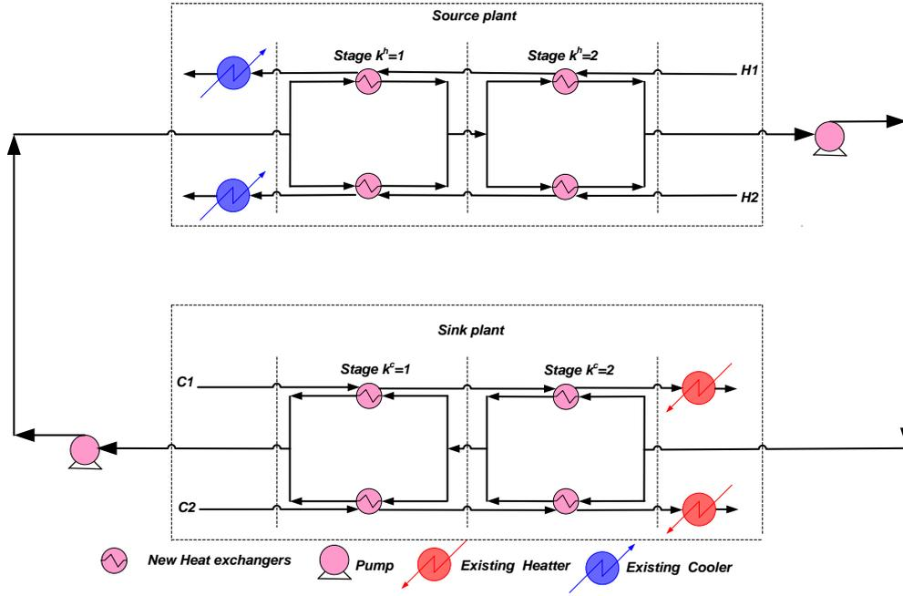
Figure 1: Superstructure of interplant Heat Integration using HRL
