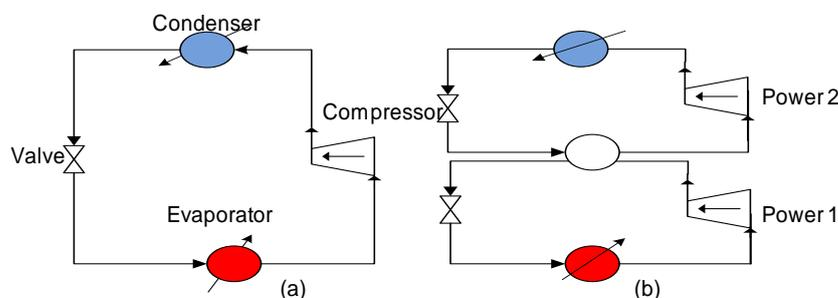
Figure 1: (a) Simple refrigeration cycle, (b) Cascaded refrigeration cycle
