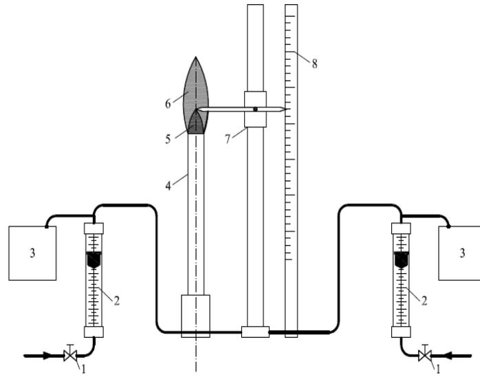
Figure 1: Laboratory stand used during the experiment (1-valves, 2-rotameters, 3-manometers, 4-burner, 5-inner combustion (kinetic) cone, 6 - outer (diffusive) combustion cone, 7-stand with a movable pointer, 8-ruler)
