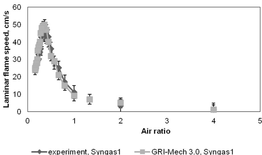
Figure 3: Laminar flame speed results – comparison of the experiment and kinetic results
