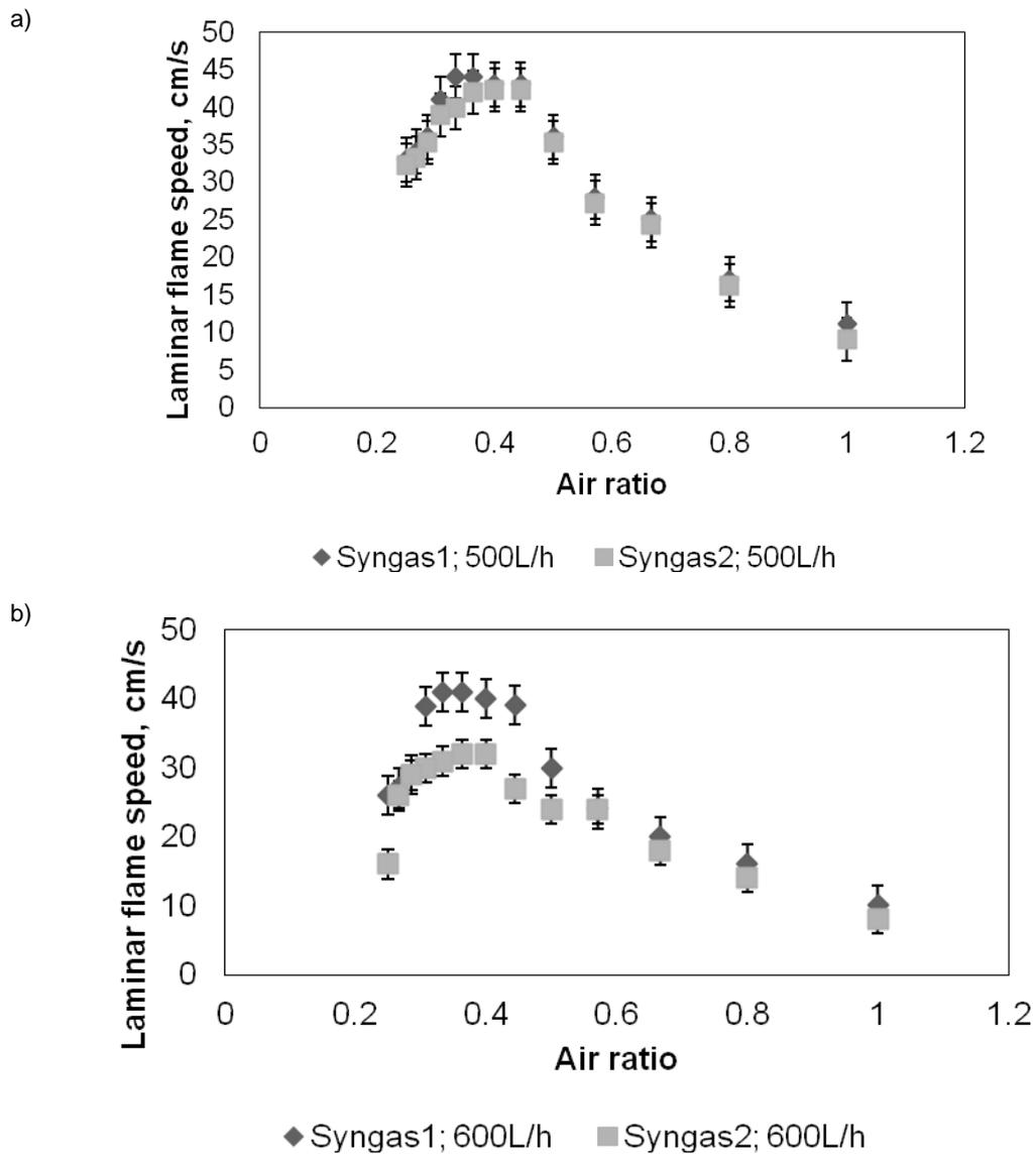
Figure 2: Laminar flame speed as a function of air ratio
