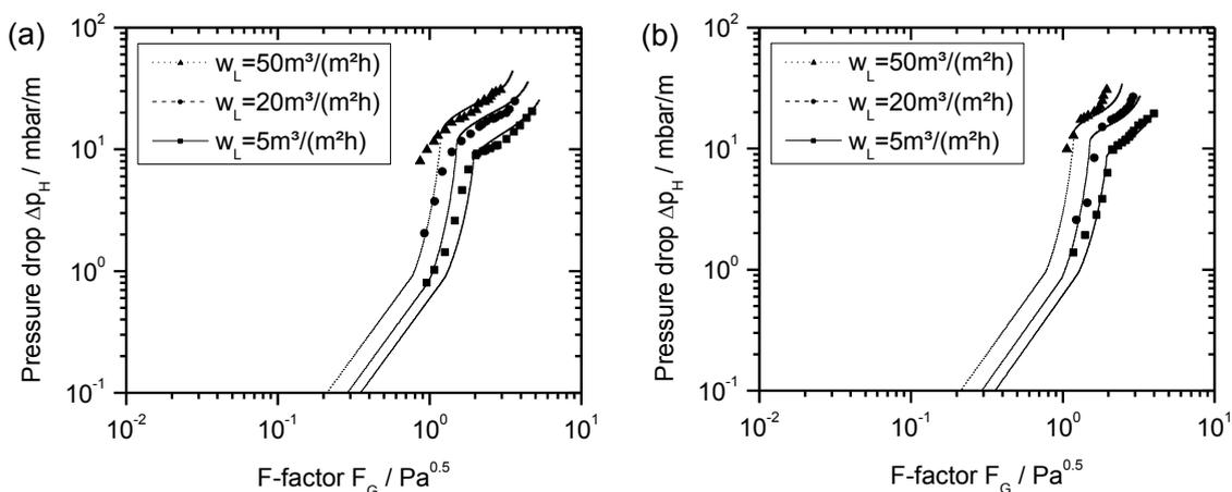
Figure 6: Comparison between simulated (lines) and experimental (points) pressure drop for B1-750T/B1-150.60 (a) and B1-750T/B1-250M (b)
