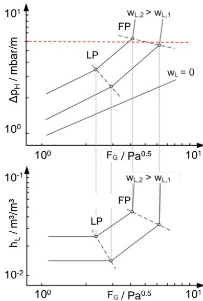
Figure 3: Typical structured packing profiles of pressure drop (above) and hold-up (below)
