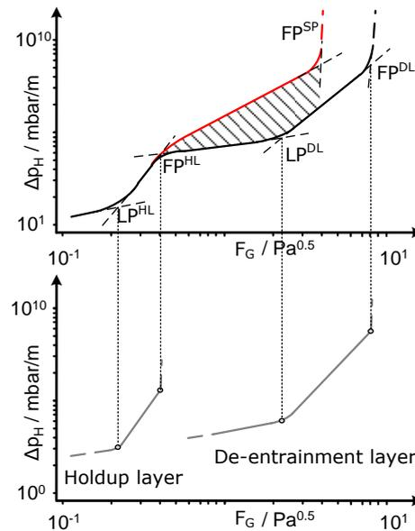
Figure 4: Pressure drop of sandwich packings (above) derived based on pressure drop of conventional packings (below)
