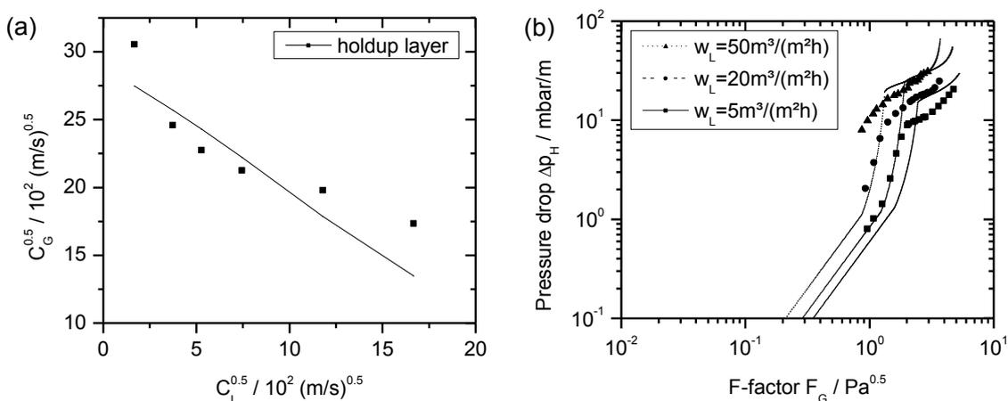
Figure 5: Comparison between simulated (lines) and experimental (points) values of capacity (hold-up layer B1-750T) (a) and pressure drop (B1-750T/B1-150.60) (b)
