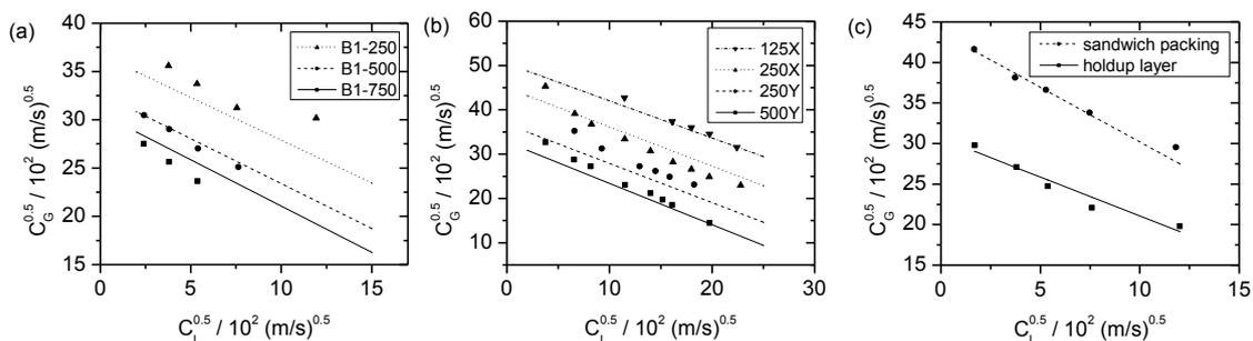
Figure 5: Wallis plot of Montz packings (a), Mellapak packings (b) and sandwich packings (c)
