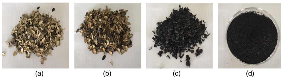
Figure 2: (a) Sunflower seed husk (SSH), (b) SSH soaked with 0.8 M K_2CO_3 ( K_2CO_3MSSH ), (c) K_2CO_3MSSH carbonized at 400 °C ( 400-K_2CO_3MSSH ) and (d) 400-K_2CO_3MSSH with particle size of 500-710 \mu m .
