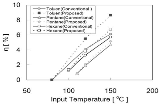
Figure 6: Comparison of power generation efficiency for different types of working fluid
