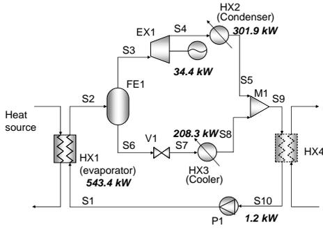
Figure 4: Conventional OFC system
