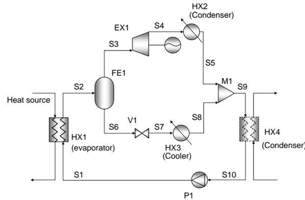
Figure 2: Conventional OFC system
