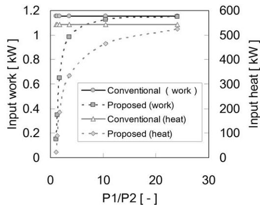
Figure 8: Input power and heat versus flash rate (working fluid: toluene, temperature in evaporator: 150 °C, temperature in condenser: 40 °C)
