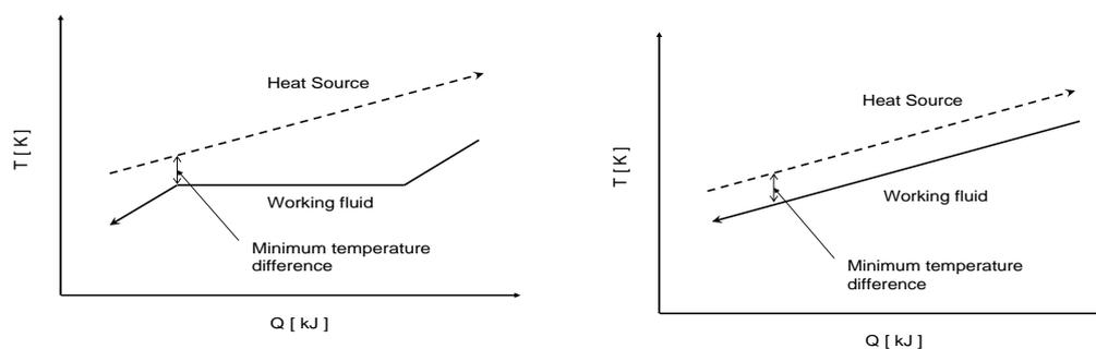
Figure 1: Temperature difference in the evaporator (left: ORC, right: OFC)
