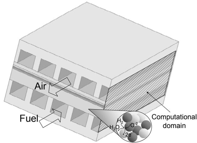
Figure 1: Schematic representation of an anode-supported SOFC
