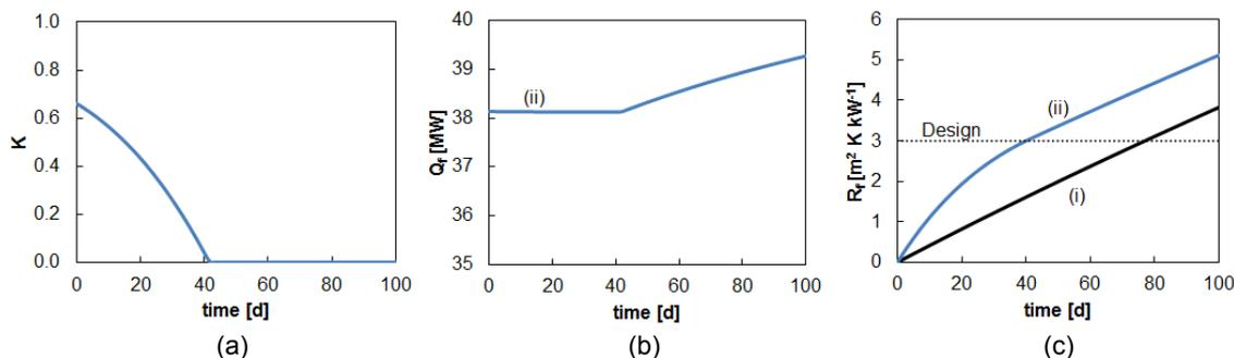
Figure 3: Bypass policy to prevent initial over-performance (Scenario ii) (a), and its impact on furnace duty (b) and fouling resistance (including comparison with Scenario (i)) (c).
