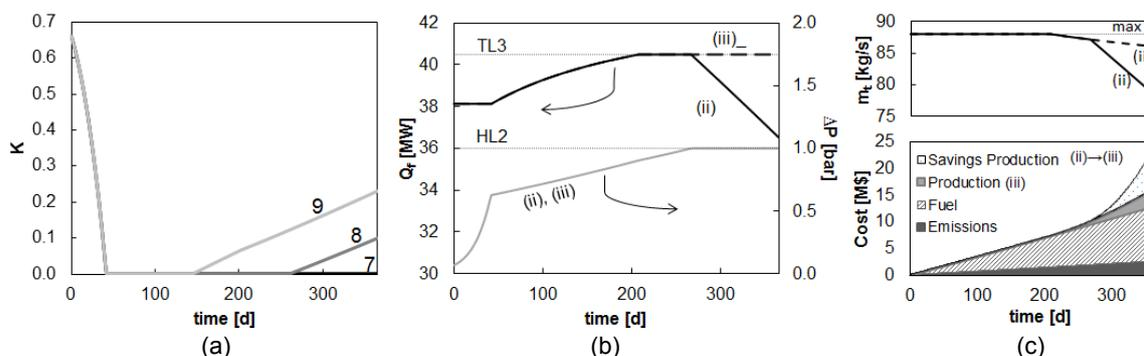
Figure 4: Bypassed fraction over time in scenario (iii) for sets THL 7-9 (a), furnace duty, pressure drop, throughput and cost for Scenarios (ii) and (iii) with THL set 8 in (b,c).
