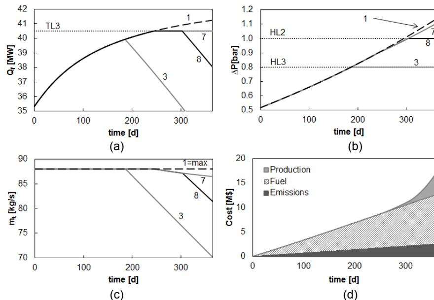
Figure 2: Evolution of furnace duty (a), pressure drop (b) and oil throughput (c) for THL sets 1, 3, 7, 8 and cumulative costs for THL 8 over a year of operation (d).
