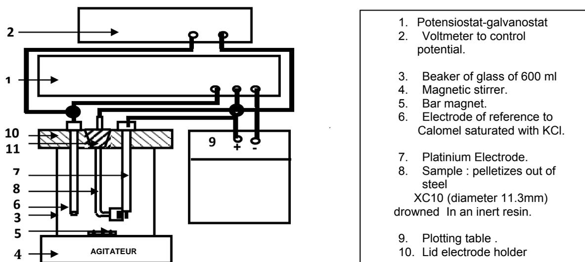
Fig.1. utilised Assembly
