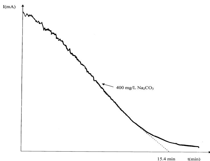
Fig.4. Curve of accelerated scaling for the water of Hamma added with 400 mg/L of  $\text{Na}_2\text{CO}_3$ .
