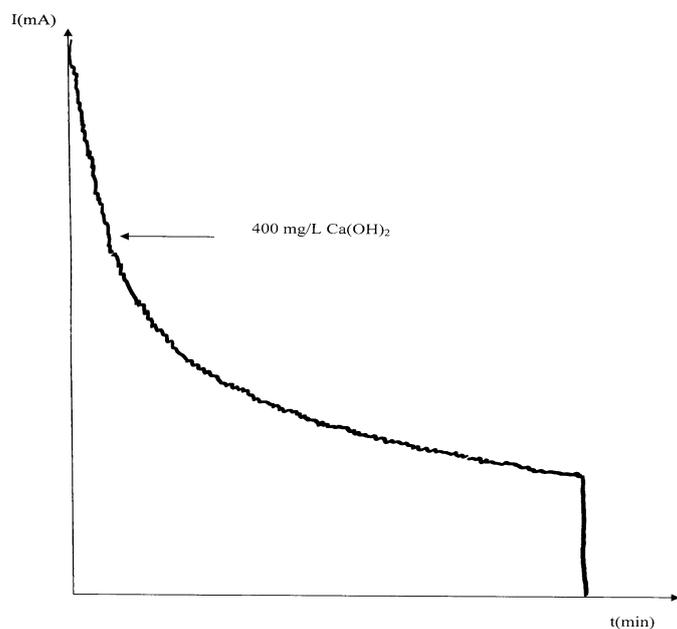
Fig.5. Curve of accelerated scaling for the water of Hamma added with 400 mg/L of lime.
