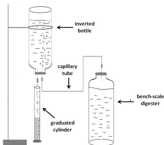
*Figure 1 - Experimental apparatus for anaerobic fermentation process and biogas measurement.*
