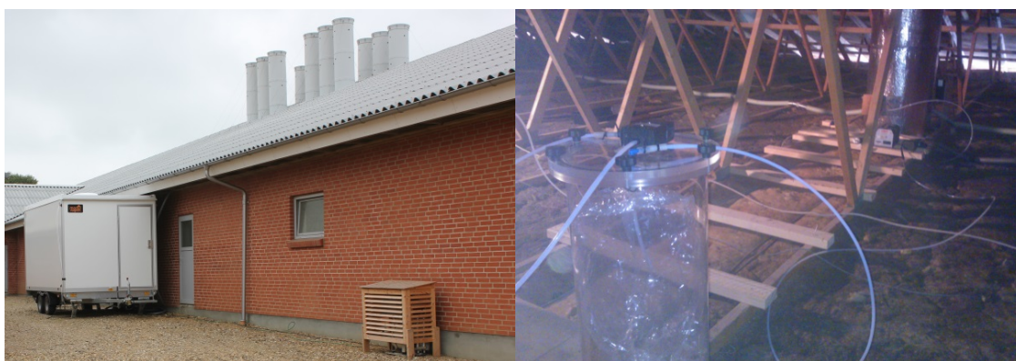
Figure 1: Left: The mobile laboratory parked next to a pig production facility, the laboratory was directly connected to the sources by isolated and heated Teflon tubes. Right: Sampling of odour bag for delayed olfactometry, the bags were connected to the sampling point with a Teflon tube.
