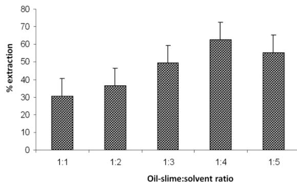
Figure 1: Influence of the solvent quantity on the degree of hydrocarbons extraction from oil-slime (chlorophorm)
