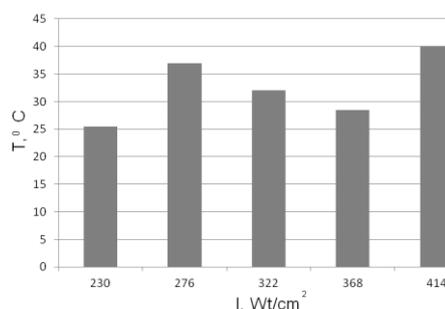
Figure 4: Influence of ultrasonic treatment intensity on the temperature of the reaction medium (extractant – chloroform)
