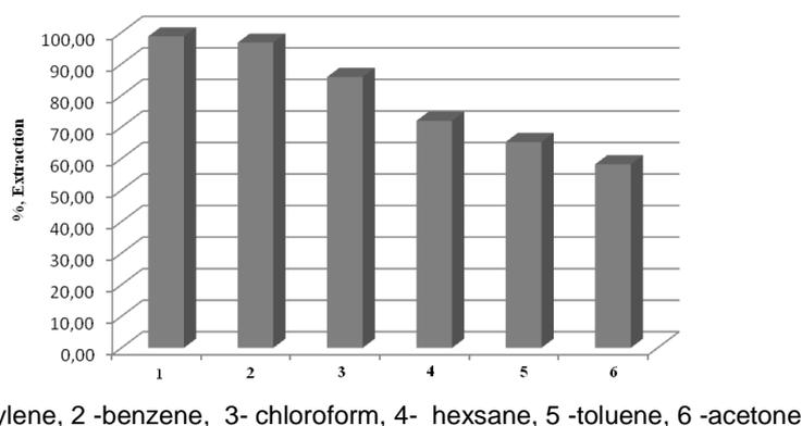
Figure 2: Extraction of oil-slime hydrocarbons with different solvents
