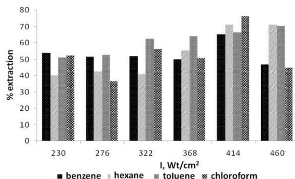
Figure 3: Influence of the intensity of oil-slime ultrasonic treatment on the degree of oil hydrocarbons extraction
