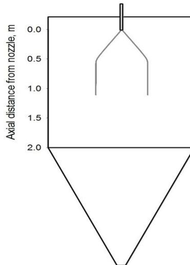
Figure 1: Trajectories of hydroxyapatite droplets in the dryer
