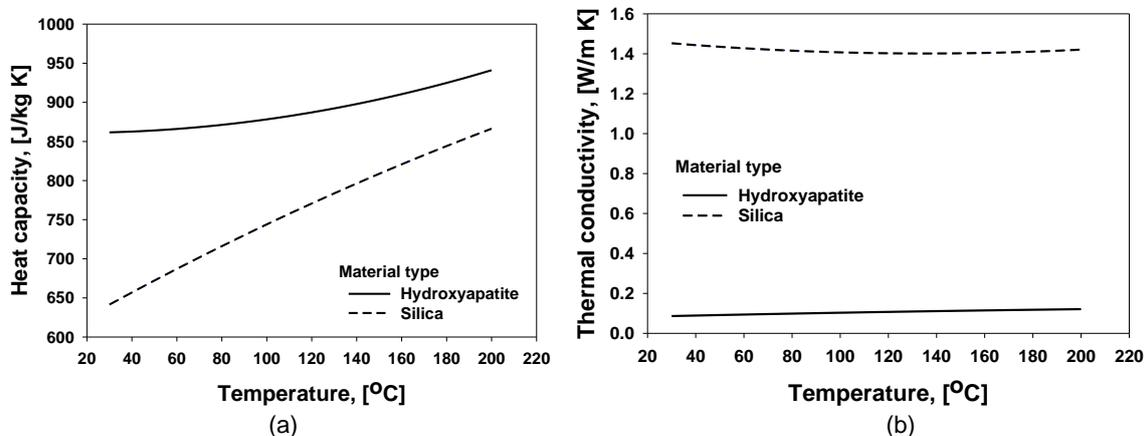
Figure 6: Temperature dependencies of (a) heat capacities and (b) thermal conductivities of hydroxyapatite and silica
