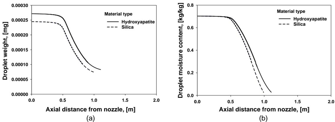
Figure 2: Profiles of (a) weight loss and (b) moisture content of hydroxyapatite and silica droplets in the axial direction of spray dryer
