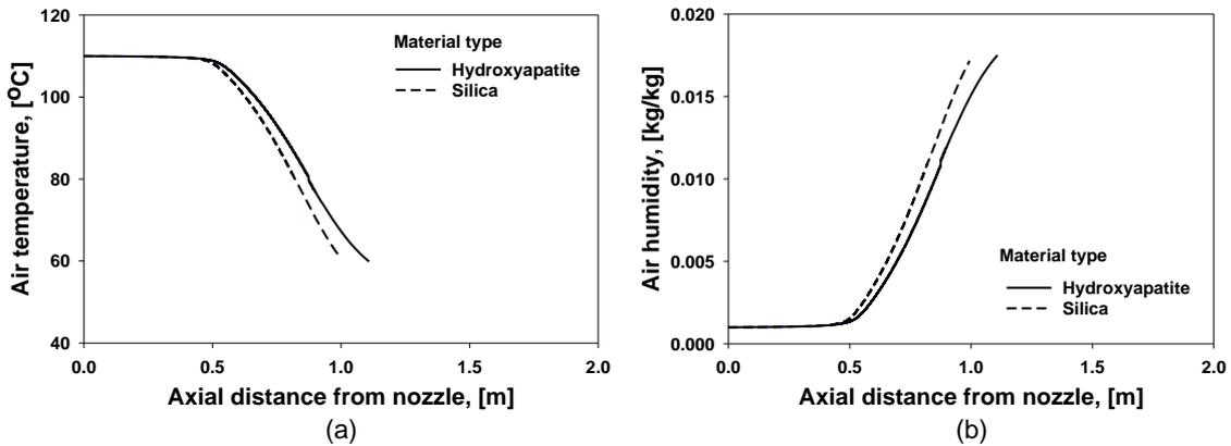
Figure 4: Profiles of air (a) temperature and (b) humidity in spray drying of hydroxyapatite and silica droplets
