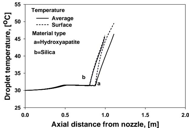
Figure 5: Profiles of average and surface temperatures of hydroxyapatite and silica droplets in spray dryer
