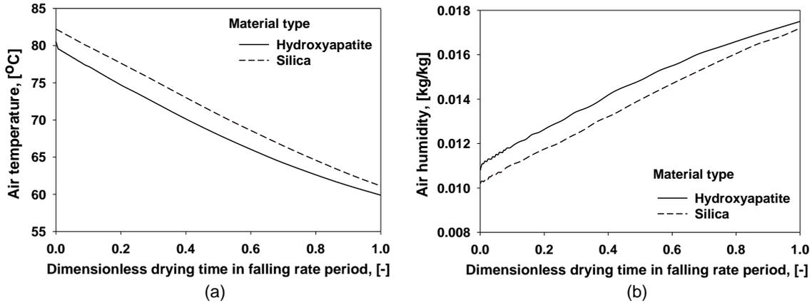
Figure 3: Variation of air (a) temperature and (b) humidity with drying time in the falling rate period
