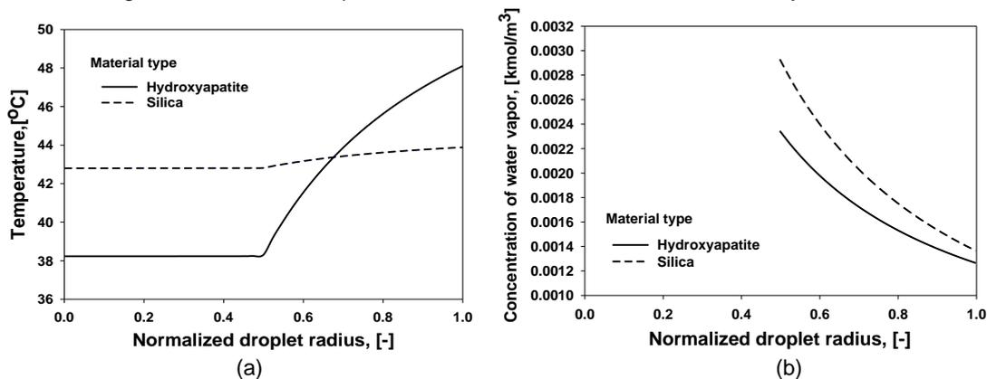
Figure 7: Distributions of (a) temperature and (b) water vapour concentration in hydroxyapatite and silica droplets
